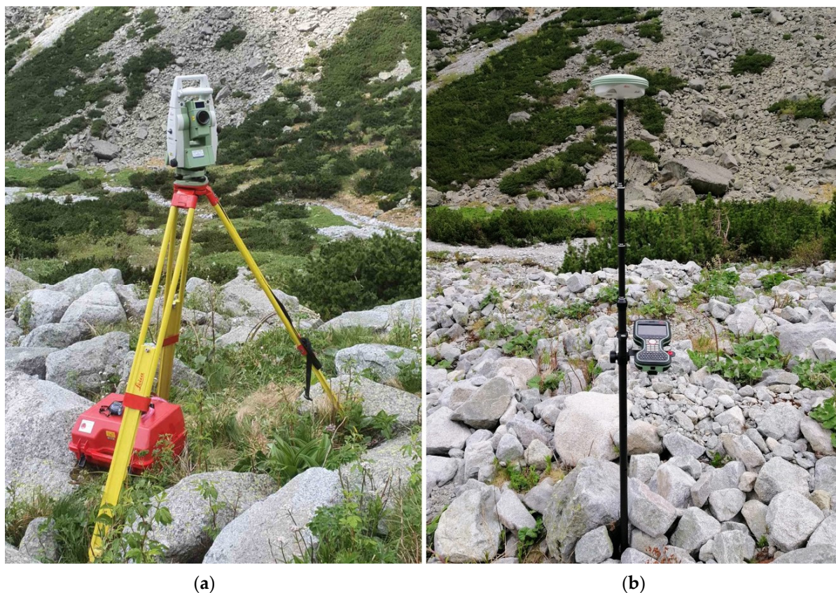
Figure 6. Total station Leica TS02 (a) and GNSS set Leica GS07 (b).
