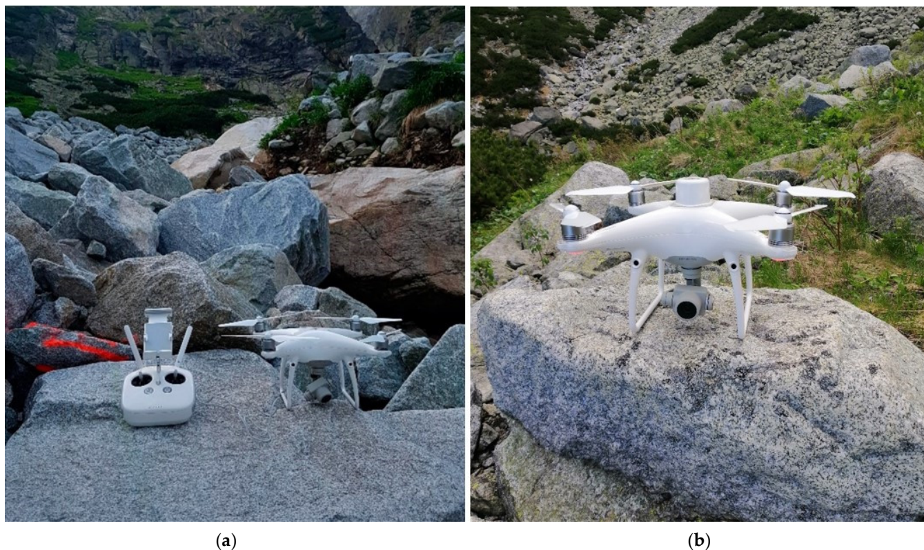
Figure 8. UAS DJI Phantom 4 Pro (a) and DJI Phantom 4 RTK (b).
