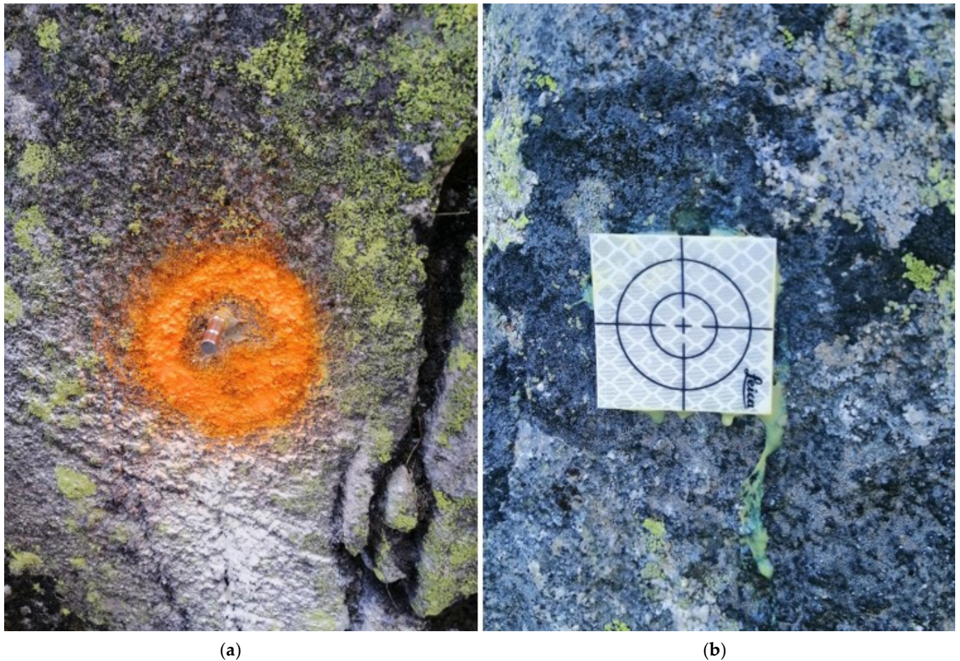
Figure 3. Stabilization of the points of the precise geodetic network (a) stainless steel pins, (b) reflective foils.
