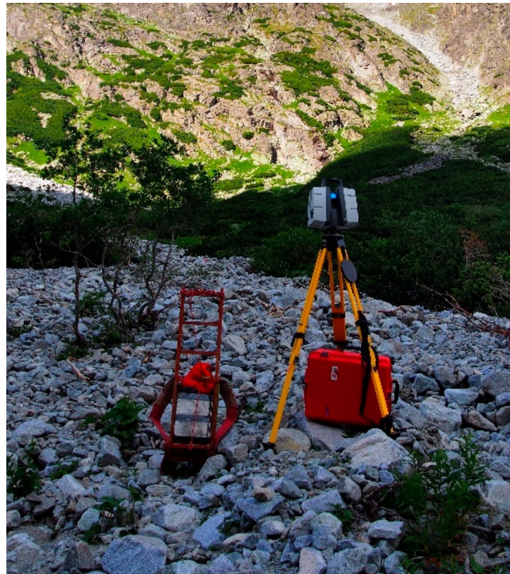
Figure 9. Three-dimensional terrestrial laser scanner Leica ScanStation P40.
