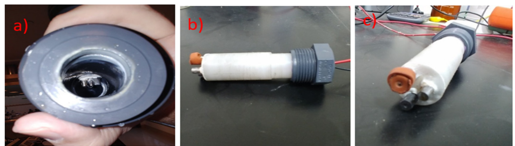
Figure 6. (a) Projection of sensor electrodes into the flow (b) isometric view of the sensor (c) side view. The orange rubber cap keeps the reference sensor (Ag/AgCl) from drying out.
