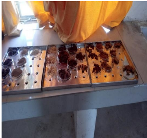
Fig. 2. Weighted Samples to be kept in oven for Moisture Estimation
