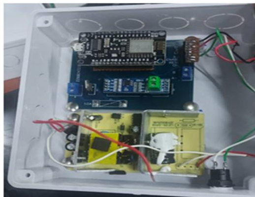
Fig. 5. An assembled IoT controller module
