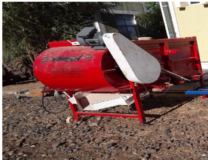
Plate 3. Multi crop seed cleaning machine
