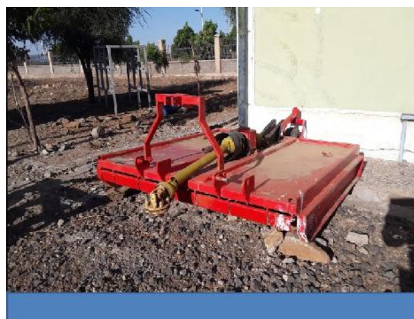
Plate 13. Rotary cutter (Crop residue and weeds cleaner)
