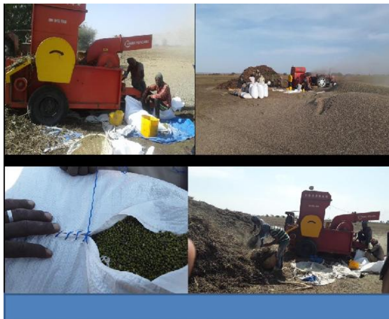
Plate 12. Mungbean threshing using multi crop thresher
