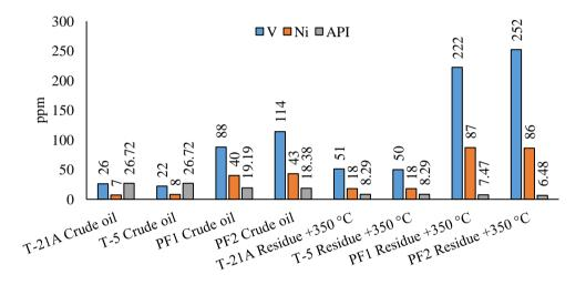
Fig. 2. Correlation of API gravity with Vanadium and Nickel content of Crude oils and Residues <sup>+</sup>350°C
