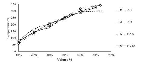
Fig. 1. Distillation Curves of T-21A, T-5, PF1 and PF2 crude oils
