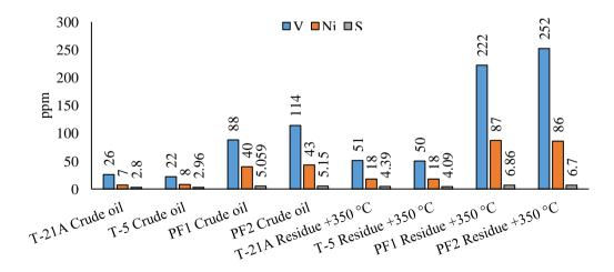
Fig. 3. Correlation of Sulfur content with Vanadium and Nickel content of Crude oils and Residues <sup>+</sup>350°C
