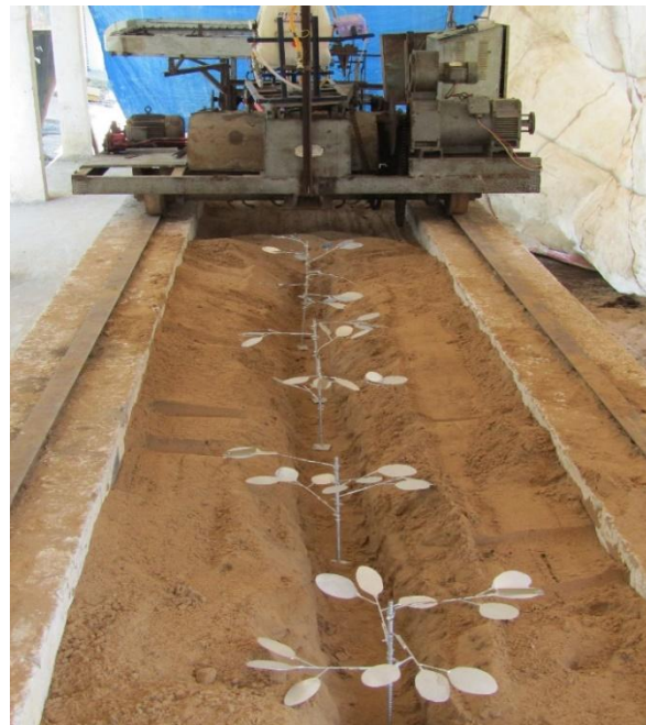
Fig. 4. Experimental setup to study effect operational parameters on droplet size of the nozzles on artificial plants
