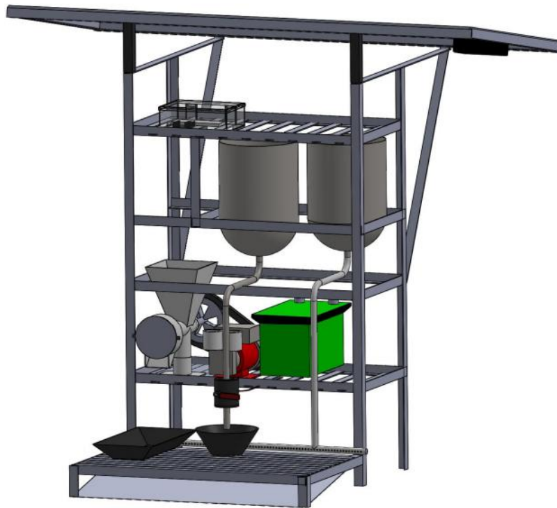
Fig. 15. Image of the management module for watering, feeding and cleaning an animal farm: three-dimensional model (3D)
