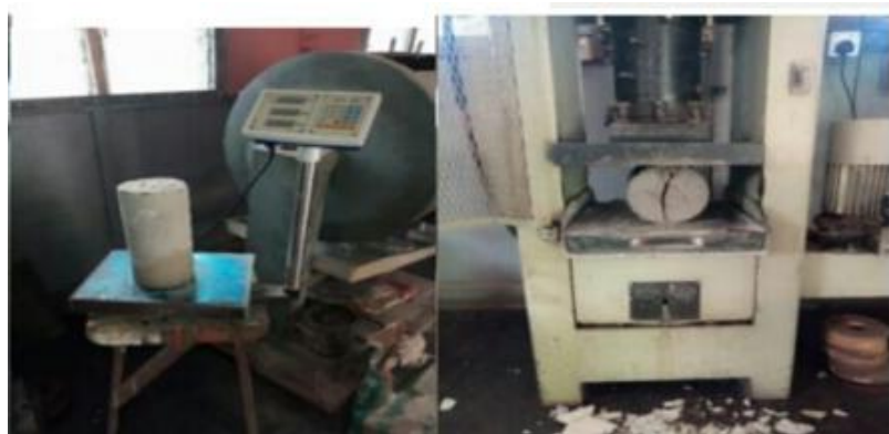
(b) Split concrete cylinder under test
