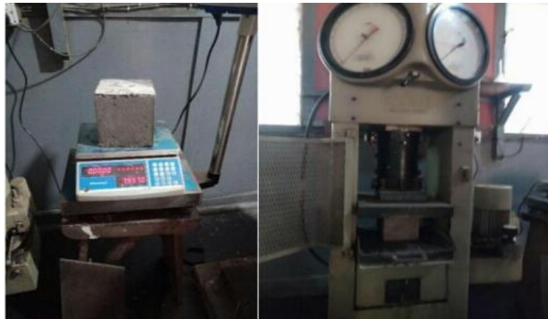
(a) Concrete cube under test
