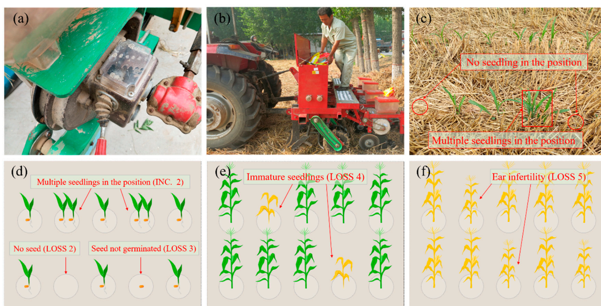
Figure 3. Seeder used and schematic diagrams of density loss. (a) The control lever used to adjust the interplant distance of the seeded; (b) the seeder in the field; (c) a representative image of seedling emergence in the field; (d–f) diagrams of LOSS 2, INCREASE 2, LOSS 3, LOSS 4 and LOSS 5. LOSS 2, LOSS 3, LOSS 4 and LOSS 5 refer to the plant density losses from TSD to ASD, ASD to ED, ED to MPD and MPD to NME, respectively. INCREASE 2 (INC. 2) refers to a plant density increase due to multiple seedlings in one position.
