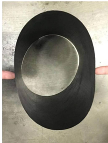
Figure 2. Cylindrical specimen deformed by touch.
