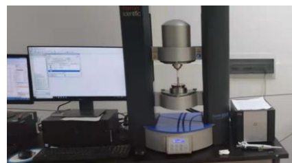
Figure 3. Haake Mars 60 rheometer used to study the rheological behavior.
