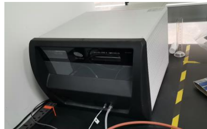
Figure 2. HotDisk TPS2500S, used to measure thermal conductivity.
