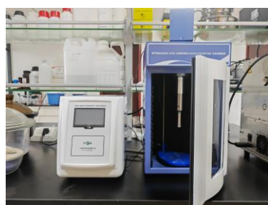
Figure 1. The ultrasonic homogenizer used in this work.
