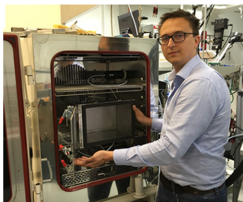
Figure 2. Calibration system fitted inside a climatic chamber.
