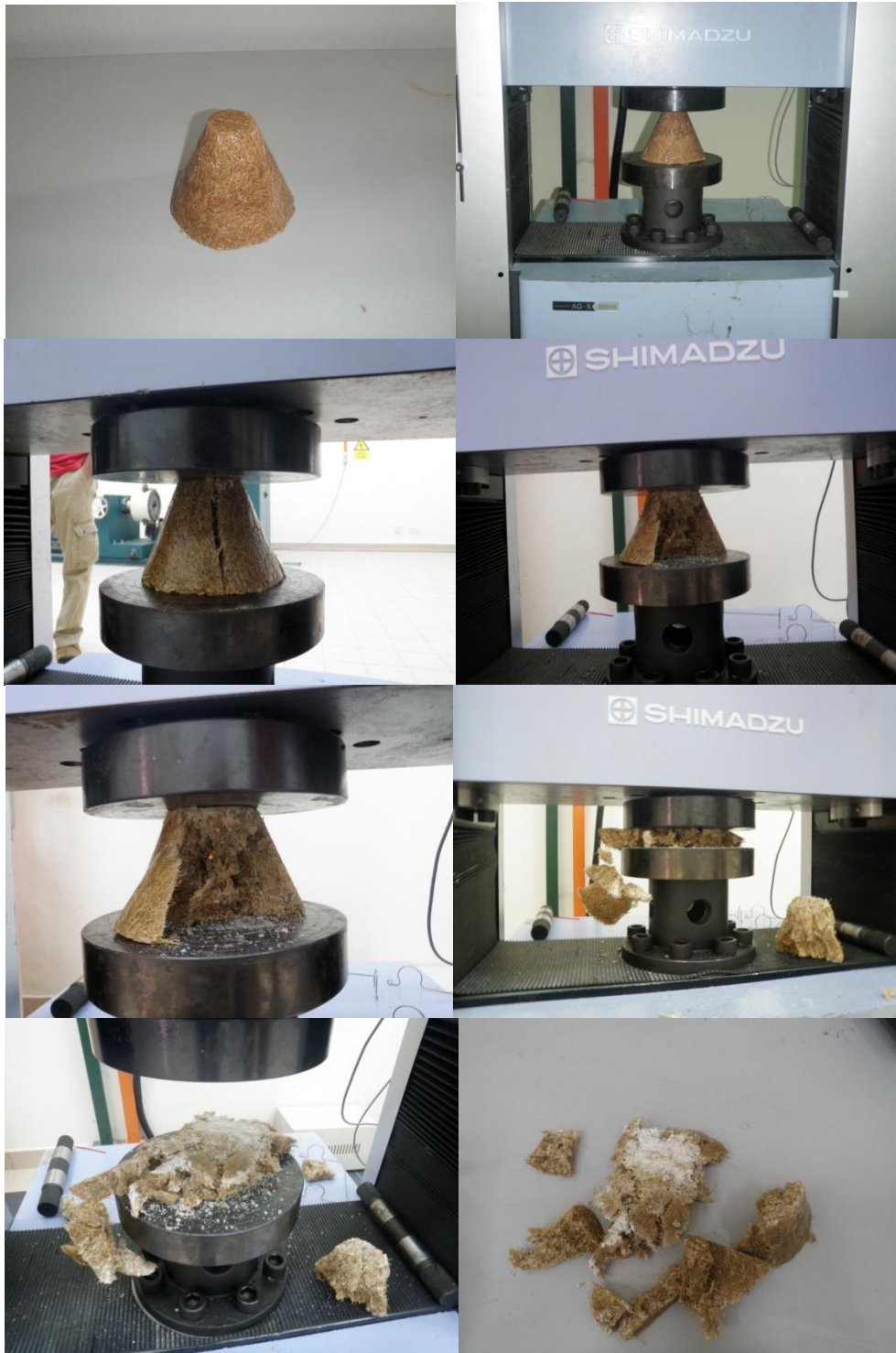
A. 1. Crushing stages of the specimens
