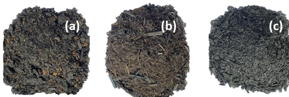
Fig. 1. Biochar produced from (a) poultry litter (b) rice straw and (c) pine wood
