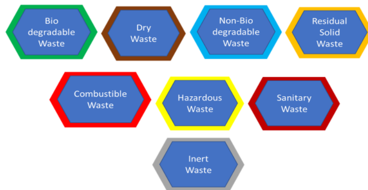
Fig. 1. Categories of solid waste as per solid waste management rules 2016 in India Source: Ministry of Environment, Forests and Climate Change, Government of India (2016 a)
