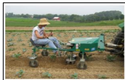
Fig. 3. ECO weeder requires an operator to move rotating weeding mechanisms with tines [24]
