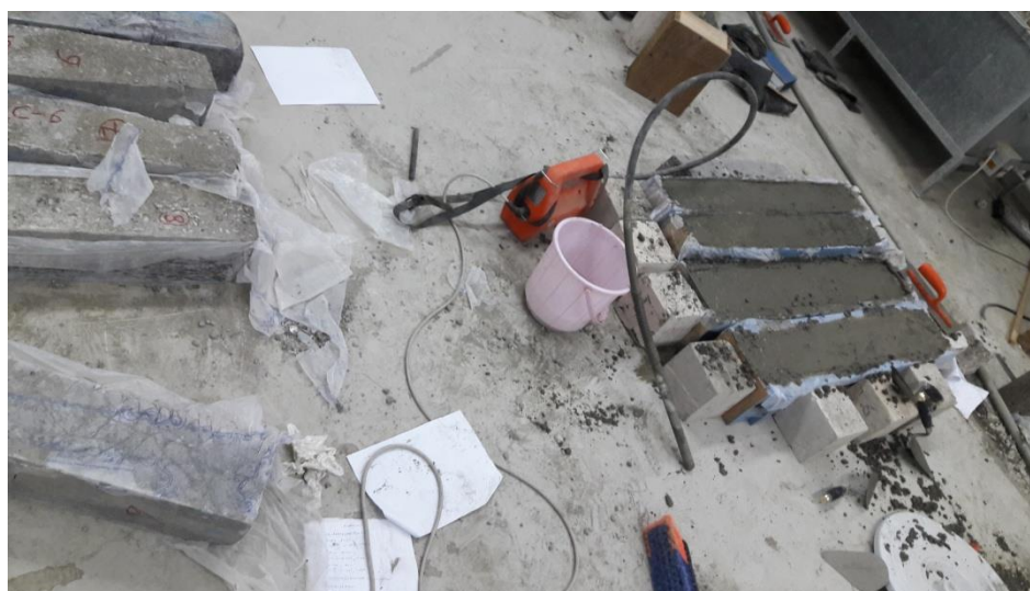
Figure 3. Controlled casting and sealed curing of concrete specimens.
